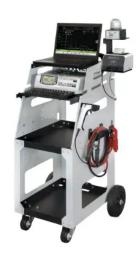
It is also able to receive software updates where there is a demand for changes in a charging curve, to meet specific vehicle manufacturer requirements. In addition, charging data can be extracted digitally.
